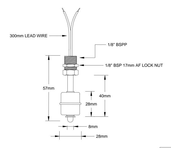
VERTICAL LEVEL SWITCH SMALL FLOAT MODEL : TC3001
